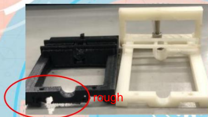
Figure 28 Comparison of slide grooves (the right side is the improved version)
