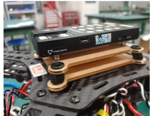
Figure 2-4 Implementation of the Newly Designed Shock Absorber Kit
