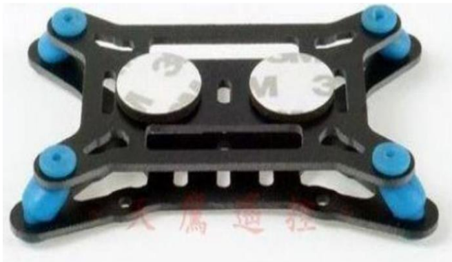
Figure 2-5 Shock-absorbing kit used last year
